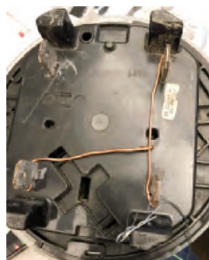
Figure 3: Bypass configuration on the back of a Form 2 meter. Both load-side terminals would be fed by the same voltage source
